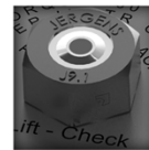
RED INDICATES LOOSE
